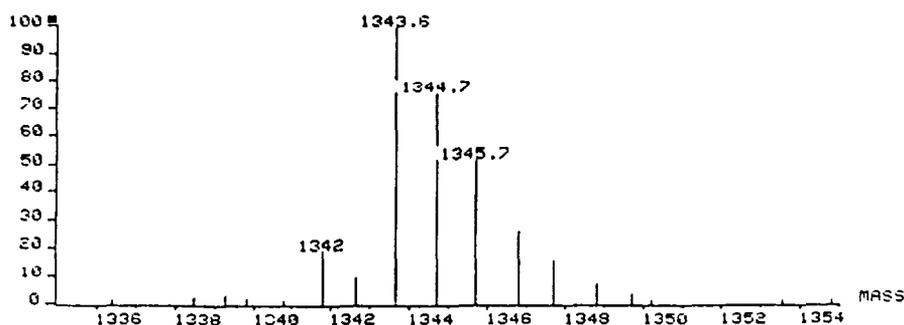
Fig. 2. FAB-MS of purified 3  $[M + H]^+$ : calculated = 1343.6, found = 1343.6.
