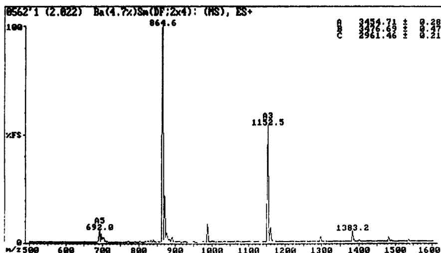
Fig. 4. ES-MS of purified **5**,  $M_+$ : calculated = 3455.1, found = 3454.7 (A), sodium adduct (B), unknown impurity (C).
