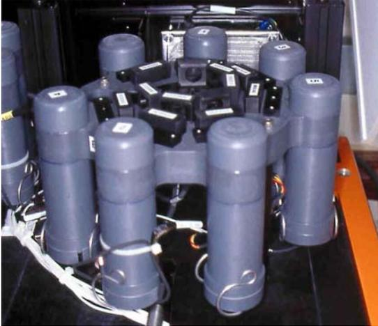
(Below). **The current default configuration for the primary PMT "octagon".** This configuration allows four-color analysis of FITC, PE, PerCP-Cy5.5 and PE-Cy7 off the primary 488 nm solid laser. The two "distal" detector slots in the signal path have no PMTs or dichroics.
